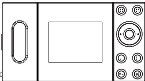
The Imago video door phone has been designed by architect Trabucco and is provided with a dedicated call loudspeaker and 3-level call tone volume adjustment (high-low-mute).
